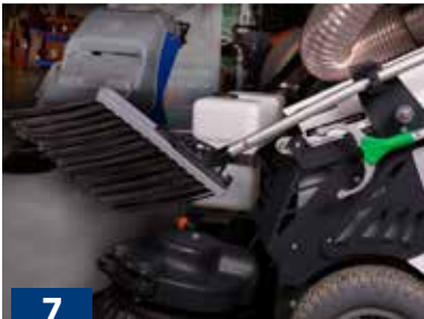
Pratico porta scope laterale Practical side broom carrier
